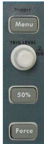
Figure 3-13 Trigger Control Zone
